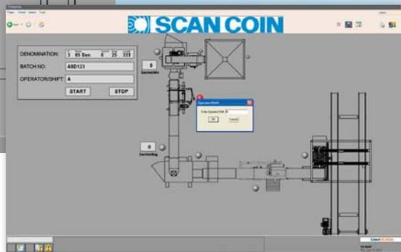
The SCAN COIN coin packaging machines have many different setup and installation options. For instance, coin blanks or minted coins can be counted and sorted in several steps, before being weighed and packed into rolls, carton boxes or sachets, finally ending up on a pallet.
